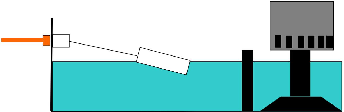
In this diagram the water level is so high that when the cooler shuts off, the water on the media can drain down into the reservoir and cause it to overflow onto the roof.
