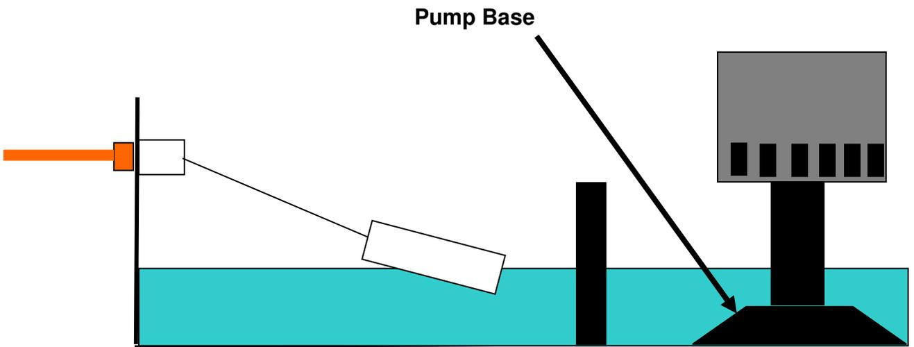
In this diagram the water level is so low that when the pump starts, the water level will fall below the base of the pump. When this happens, the pumps capacity drops by half or more.
