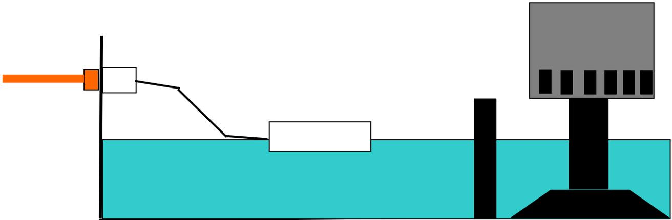
By putting a step in the arm of the float, it allows the valve to travel open and closed faster with less change in the water level. By using a pair of pliers to hold the float arm, it can be bent in this fashion.
