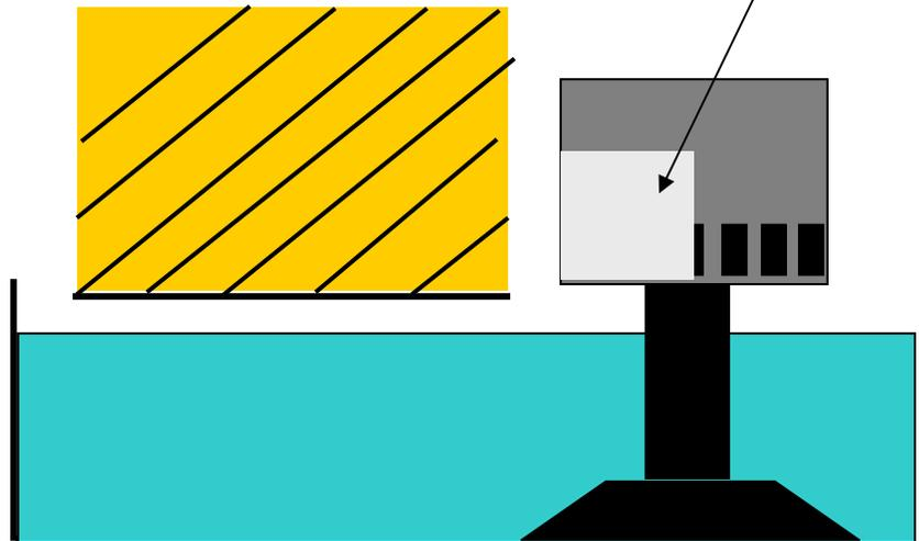
Adjusting the float valve so as to get enough water to cover the base of the pump but not overflow on shutdown can be difficult.
